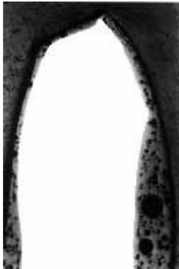
Direct-on white enamelling on a squeezed-off edge (50 : 1)
