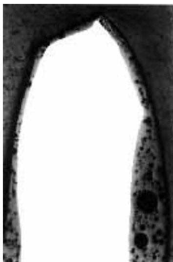
Direct-on white enamelling on a squeezed-off edge (50 : 1)
