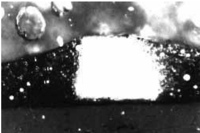
Sulphate dimple (cross section)
