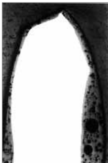
Direct-on white enamelling on a squeezed-off edge (50 : 1)
